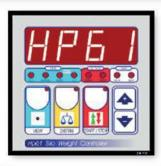
It figures actual weight of the silo and manage to deliver to any hopper inside the house.
